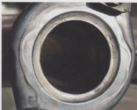
Fig. 2: Pipe/flange joint brazed with a CrNi alloy (sources: TU Dresden and eldec).
