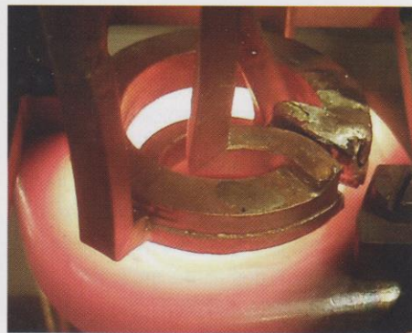
Fig. 1: High-temperature shielding gas brazing of a special flange with a pipe using an outer field inductor with an integrated shielding gas shower (sources: TU Dresden and eldec).
