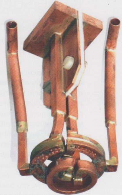
Fig. 4: Two-turn ring inductor with a shielding gas shower device.
